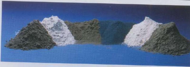
Figure 2: Fly Ash, Slag and Silica Fume offer environmental and Performance benefits when optimally combined with portland cement in concrete mix designs (Source: America's Cement Manufacturers (2015); Using Concrete as a Sustainable Solution for Buildings)
