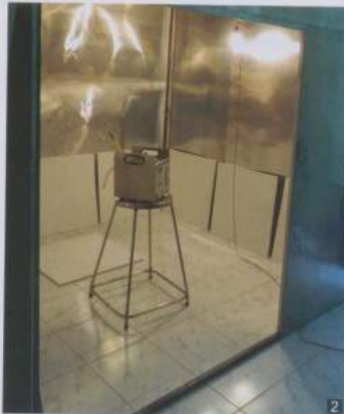
2. Experimental chamber to measure VOC emissions
