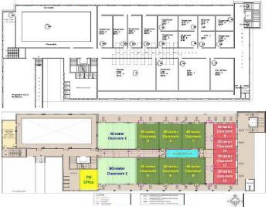
Figure 1: Spatial layout before and after retrofit
